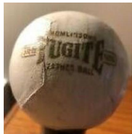
The advent of synthetic surfaces rang the death knell for the leather ball. On water-based surfaces, the leather case absorbed water and became swollen. It was like hitting a sodden ball of wool. Hockey Australia asked Kookaburra to develop a ball suitable for play on synthetic surfaces. This was in 1982 and the Kookaburra dimpled ball has been used in every Olympic Games and virtually all other international tournaments since 1984.
